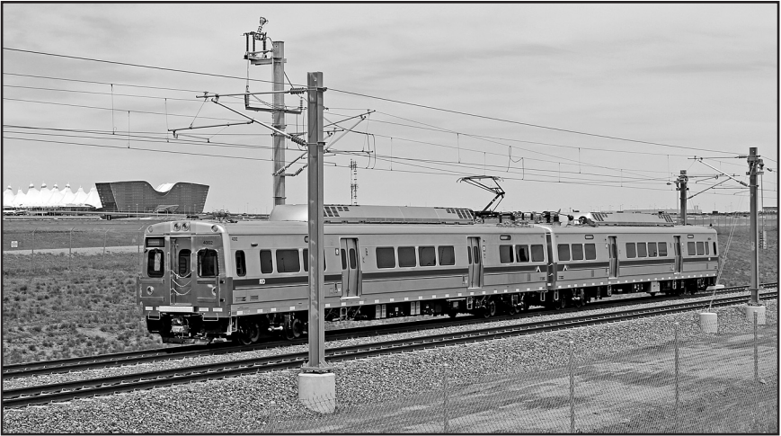
RTD commuter cars 4002 & 4001 test running under live wire at Denver International Airport on May 12, 2015. The track ends at the new hotel on the south end of the terminal (visible above the front of the left unit). – Photo © 2015 Dave Schaaf.
